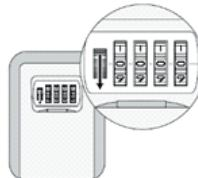
3. Press down the key safe opening switch to open it.
