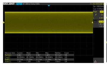
SDS1004X-U can measure all sampled data points up to 14 Mpts. This ensures the accuracy of measurements while the math co-processor decreases measurement time and increases ease-of-use.
