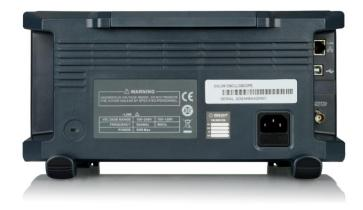
SDS1000X-U supports USB Host, USB Device (USB-TMC), LAN (VXI-11), Pass/Fail and Trigger Out
