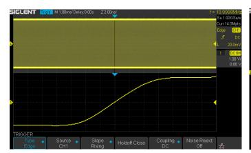
Using hardware-based Zoom technologies and max record length of up to 14 Mpts, users are able to oversample to capture for longer time periods at higher resolution and use the zoom feature to see more details within each signal.
