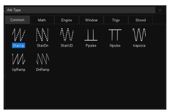
The built-in waveform generator can output waveforms with up to 25 MHz frequency and  $\pm 3$  V amplitude. Six basic waveforms together with multiple types of predefined waveforms and as user-defined arbitrary waveforms are supported.
