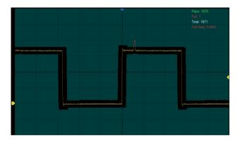
The SDS5000X utilizes a hardware-based Mask Test function, performing up to 18,000 Pass / Fail decisions each second. It is easy to generate user-defined test templates in order to provide trace mask comparisons, making it suitable for long-term signal monitoring or automated production line testing
