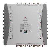
Cascade multiswitch for 4 Satellite positions with 17 inputs and 17 trunk outputs, suitable for distributing satellite and terrestrial signals in small to large sized systems. Available with 24 subscriber outputs and powered by the TMS PSU external power supply either directly or via the SAT trunk lines.
