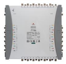
Cascade multiswitch for 3 Satellite positions with 13 inputs and 13 trunk outputs, suitable for distributing satellite and terrestrial signals in small to large sized systems. Available with 24 subscriber outputs and powered by the TMS PSU external power supply either directly or via the SAT trunk lines.
