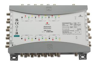
Cascade multiswitch for 3 Satellite positions with 13 inputs and 13 trunk outputs, suitable for distributing satellite and terrestrial signals in small to large sized systems. Available with 16 subscriber outputs and powered by the TMS PSU external power supply either directly or via the SAT trunk lines.
