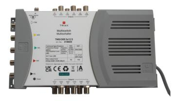
Standalone multiswitch for 1 Satellite position with 5 inputs and 12 outputs, suitable for distributing satellite and terrestrial signals in small and medium sized systems.
