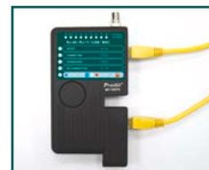
RJ45 LAN cable test
