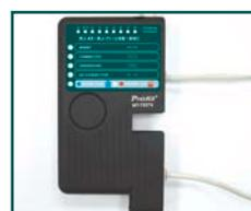
RJ11/12 telephone wire test
