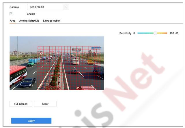
Figure 11-3 Set Motion Detection
