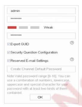
Figure 2-1 Activate the Device
