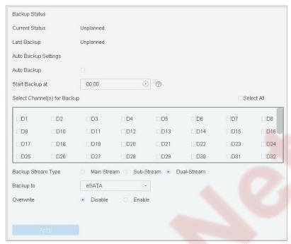
Figure 7-4 Configure eSATA for Auto Backup
