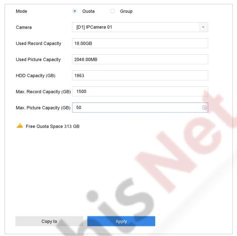
Figure 7-8 Storage Mode-HDD Quota
