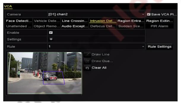
Figure 9-8 Draw Area for Intrusion Detection
