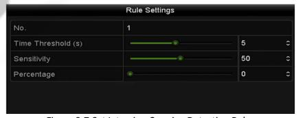
Figure 9-7 Set Intrusion Crossing Detection Rules
