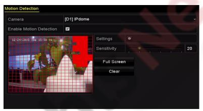
Figure 5-11 Motion Detection
