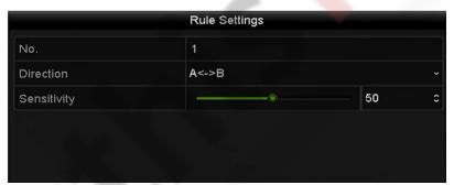
Figure 9-5 Set Line Crossing Detection Rules
