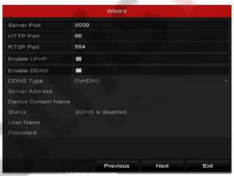
Figure 2-20 Advanced Network Parameters
