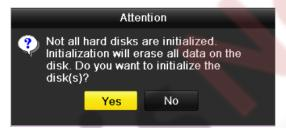
Figure 12-1 Message Box of Uninitialized HDD
