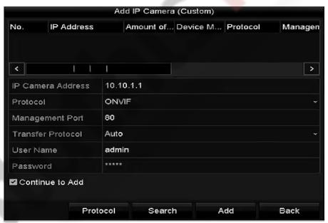
Figure 2-31 Custom Adding IP Camera Interface
