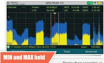
Display them separately or simultaneously along with the current spectrum trace.
