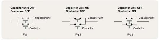
Note) Closing sequence: Fig.1 => Fig.2 => Fig.3 Opening sequence: Fig.3 => Fig.1
