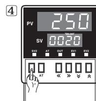
Push MD key when the setting is completed. It will stop flashing, then return to **RUN** mode.
