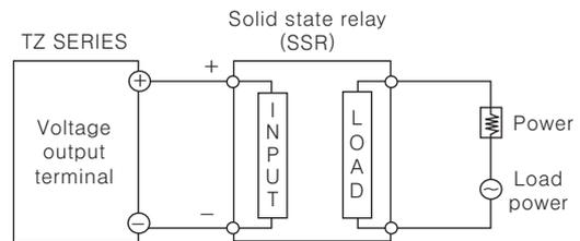
※SSR should be selected by the capacity of load, otherwise, it may short-circuit and result in a fire. Indirect heated should be used with SSR for efficient working.
