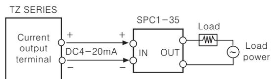
※It is important to select SCR unit after checking the capacity of the load.
