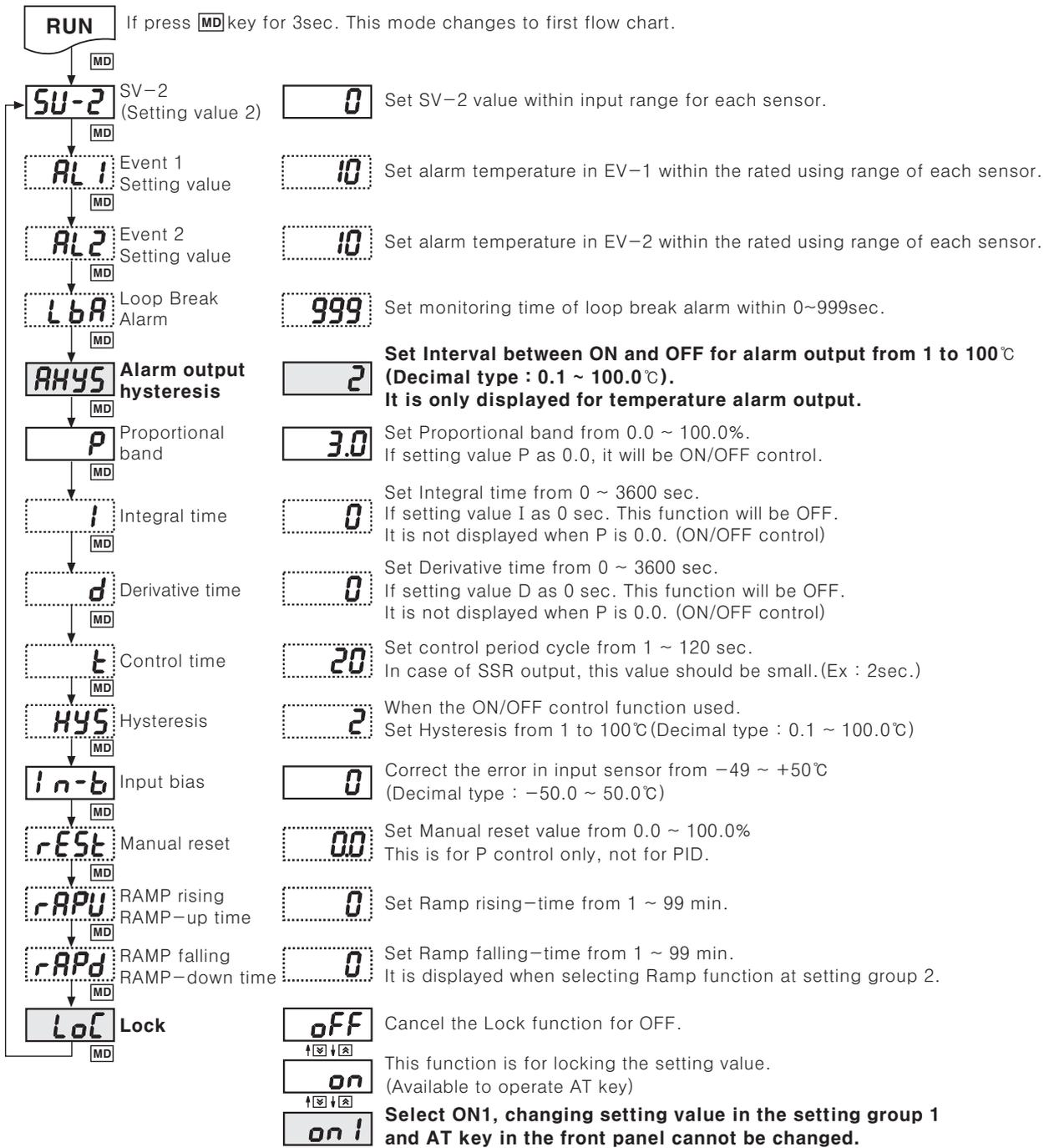
※ It will start to flash by pressing **◀** (◀) key and the flash will be moved by **◀** (◀◀), **▶** (▶▶) keys then set the value by **▲** (▲), **▼** (▼) keys. After that if pressing **MD** key the DATA will be changed then display next mode.
