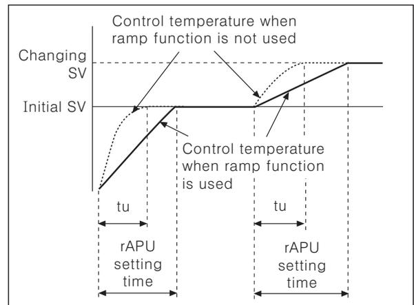
It makes delay rising temperature when change the set value at stable control status or delay the initial rising temperature as like above picture.
