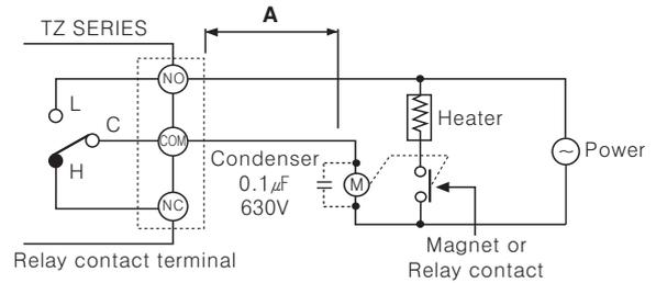
Keep power relay as far away as possible from TZ/TZN series. If wires length of **A** is short, electromotive force occurred from a coil of magnet switch & power relay may flow in power line of the unit, it may cause malfunction. If wires length of **A** is short, please connect a mylar condenser 104 (630V) across coil of the power relay "M" to protect electromotive force.
