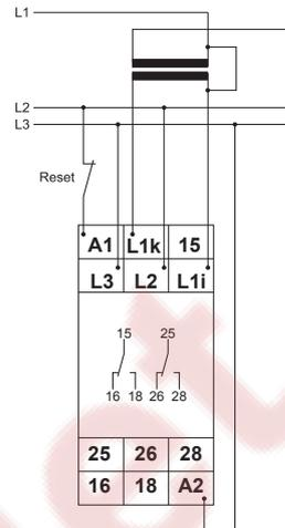
Connected to 1~ 230V mains with power module 230V a.c. without fault latch
