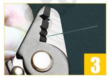
Strips the 250µm cable down to the glass fiber without nicks or scratches.
