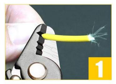
Strips the 1.6-3.0mm fiber jacket down to the 600-900 µm buffer coating
