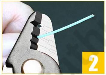
Strips the 600~900µm buffer coating down to the 250µm coating.
