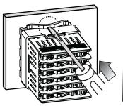
\*Insert product into a panel, fasten bracket by pushing with tools as shown above
