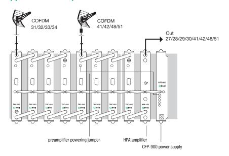
Exemple of «TPC» headend for conversion of four digital channels and processing of other four ones. Contains 8 TPC-010 Processors, 1 Amplifier and 1 Power Supply, all fixed on 2 horizontally joined Baseplates.
