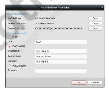
Figure 2-9 Modifying the Network Parameters
