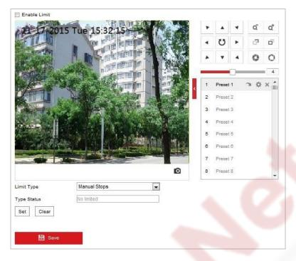
Figure 5-28 Configure the PTZ Limit
