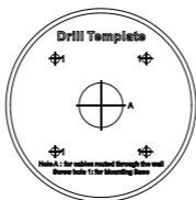
Figure 2-13 Drill Template of the Junction Box
