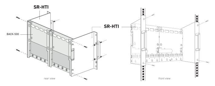
Rack 19" fixing for two base-plates (BACK-500) headend installation
