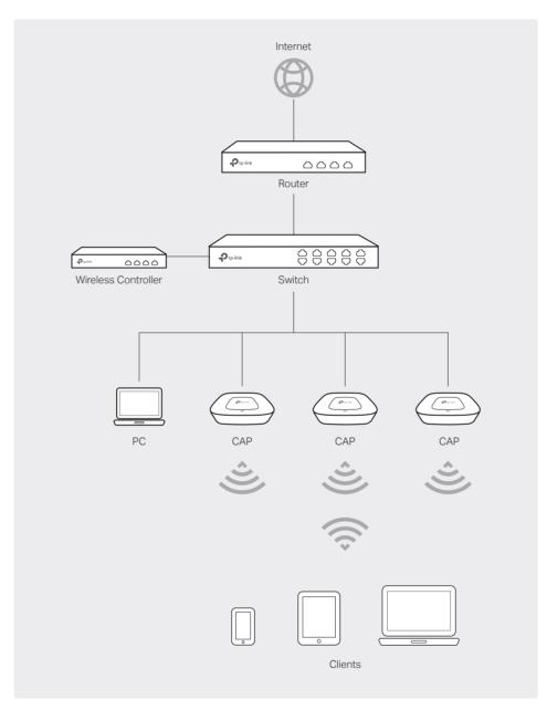
$\bullet$  The wireless controller can be in the same or different network segment as the CAPs.
