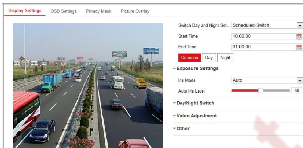
Figure 9-5 Day/Night Scheduled-Switch Configuration Interface
