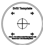
Figure 2-12 Drill Template of the Junction Box
