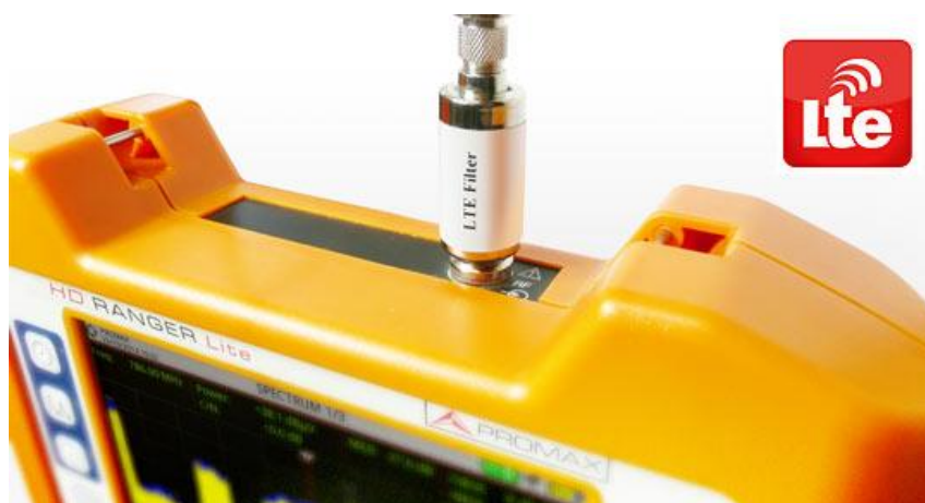
Figure A5.6 LTE filter coupled to a HD RANGER Eco field strength meter.
